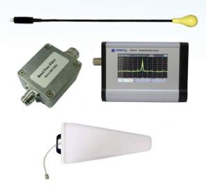
Cell Sites are naturally rich with joints of different metals, and at some conditions these passive junctions behave as non-linear devices, hence generating what's called InterModulation. Any 2 signals can hit such elements and generate IM products which interfere with another co-existing channel at the same site or nearby. Hence, passive intermodulation is a critical issue in cellular networks and despite its relatively small level, it has serious effects if not mitigated.
