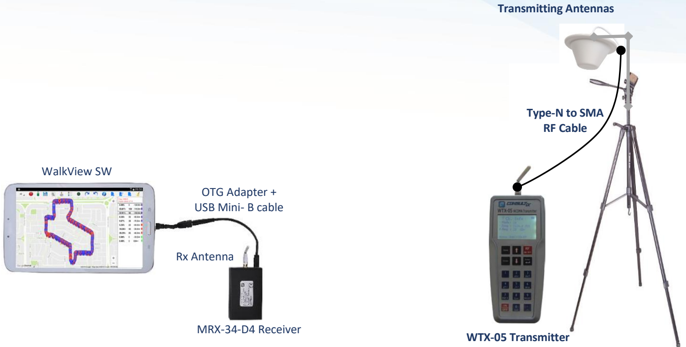
Figure 15: Typical Walk Test Setup
