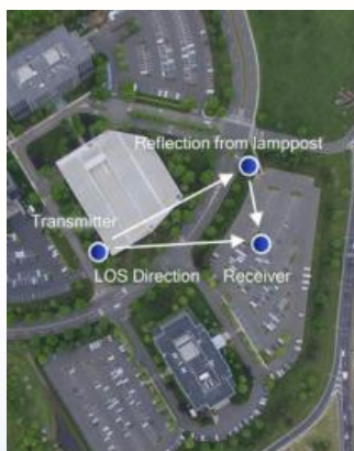
Figure 3a. TX RX arrangements
