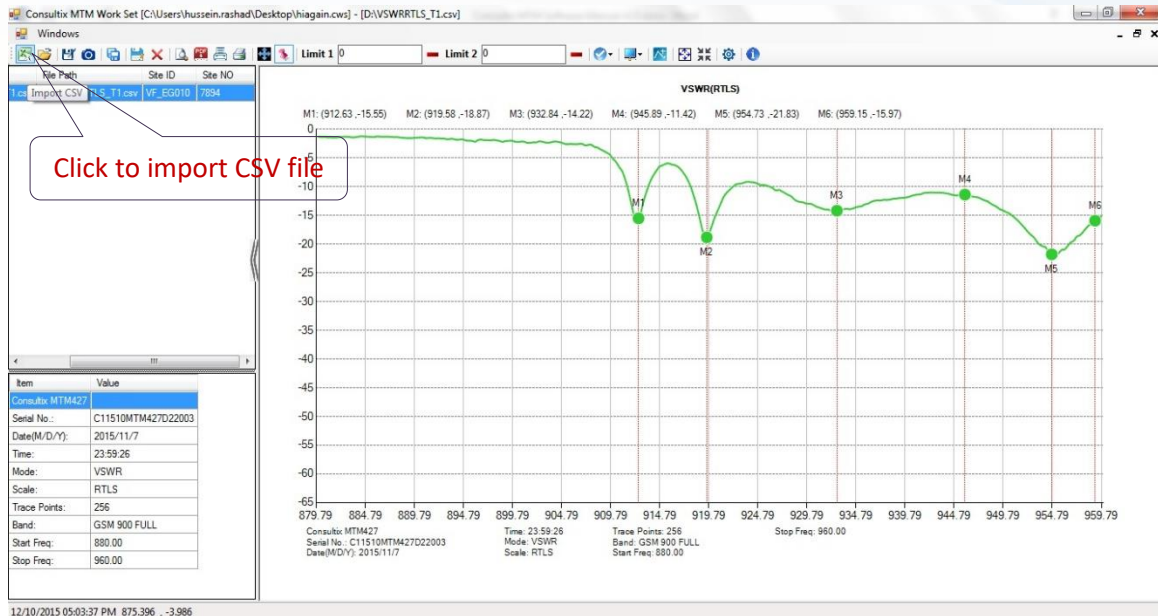
Figure 2, VSWR-Return Loss measurement trace
