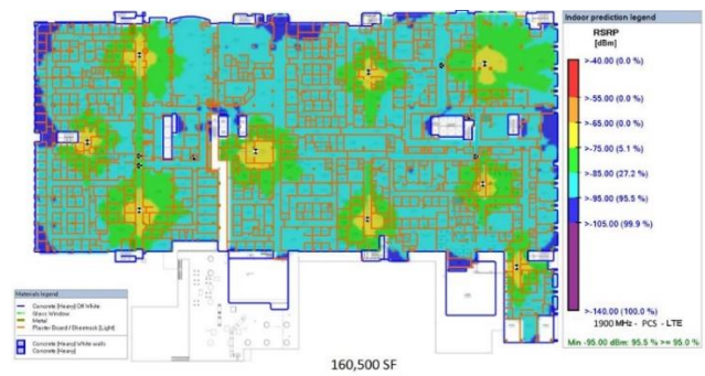
Figure 8. Wall type Sheet rock-Light (incorrect Passing)
